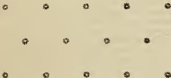
the objects in the alternate rows "breaking joint" with those in the others, and the rows being placed at such a distance apart that the distances between any object and those lying around it are all equal.
